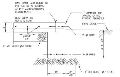
NOTE: CONNECTION DETAILS OF BUILDING SKID TO CONCRETE SHOULD BE USED AS A GUIDELINE. CONTRACTOR SHALL FOLLOW PRE-FAB METAL BUILDING MANUFACTURER'S RECOMMENDATIONS FOR CONNECTION OF BUILDING SKID TO CAST-IN-PLACE CONCRETE SLAB.
